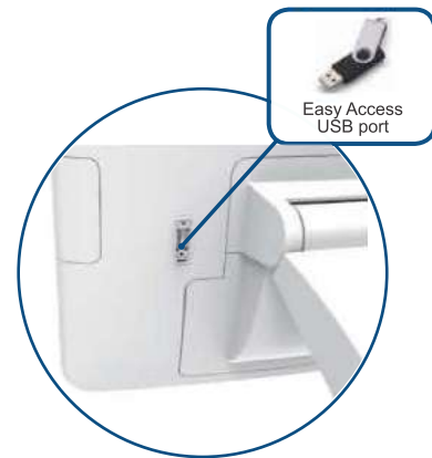
Easy Access USB port 1xUSB port on backside w/ rubber cover for USB port to ensure data security (Optional) Screwed bracket design
